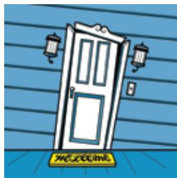
Uneven spaces around doors and windows can indicate shifting of the foundation.
