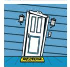
Uneven spaces around doors and windows can indicate shifting of the foundation.
